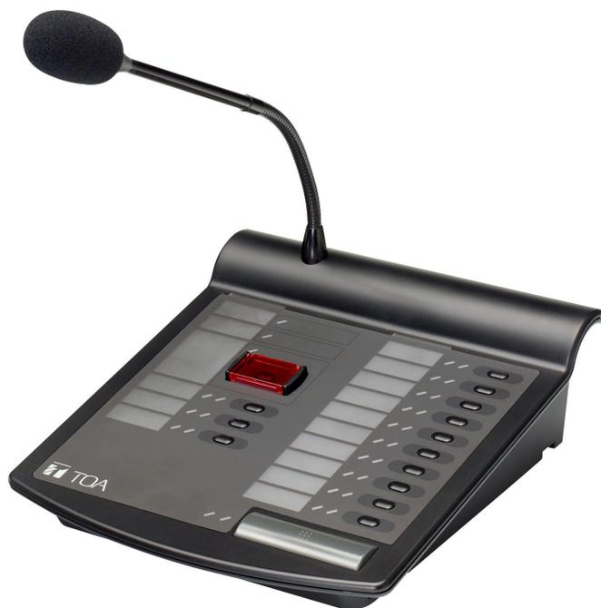
VX-100RM-EA is an IP PoE Remote Microphone. VX-100RM-EA Remote Microphone is used for general and emergency broadcast. It is equipped with 10 function switches that can be used to select individual zones or zone groups a covered switch and corresponding indicators. The optional RM-110VX-EA Remote microphone extension permits switches and indications to be expanded in 10-piece units.
