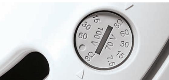
Control 47CT, 47LP, 47HC and 40CS/T provide low-saturation transformers for use on 70V/100V distributed line, switchable for 8Ω bypass.
