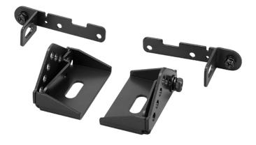
The HY-WM2B is used exclusively to mount the HX-5 series speaker system closely to a wall or ceiling. The bracket helps to achieve clearer sound reproduction by minimizing phase interference generated by sound waves reflecting from walls or ceilings. This bracket is designed for indoor use.
