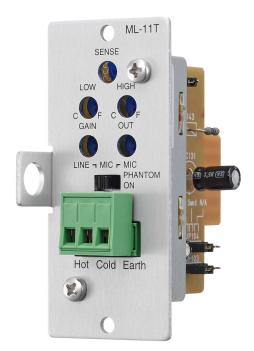
The ML-11T is a Microphone/Line input module with a mute send/receive designed for use with 900 Series amplifiers. Phantom power is provided for condenser microphone use.
