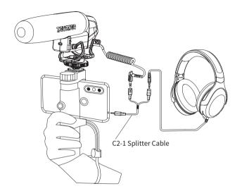
5. When connecting with camera or DSLR for recording, it is recommended to set the mic volume fader to 0dB. When connecting with cell phone for recording, it is recommended to set the mic volume fader to +10dB.
