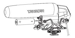
2. When assembling it with camera or DSLR, insert the cold shoe into the slot of the camera. Turn the knob clockwise to fix the microphone. When assembling it with photography stand, connect the 1/4 socket on the microphone with photography stand. Turn it clockwise to fix the microphone.
