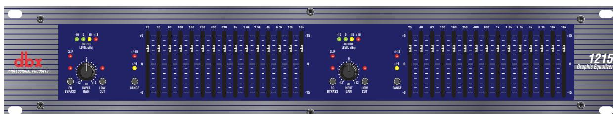
**Input Gain Control:** This control sets the signal level to the equalizer. It is capable of -12dB to +12dB of gain. Its effect is apparent by viewing the OUTPUT LEVEL BAR GRAPH.
