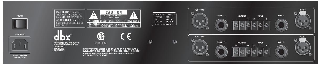
**Power Switch:** Switches the power on and off. Always make audio connections with the power switch in the OFF position.
