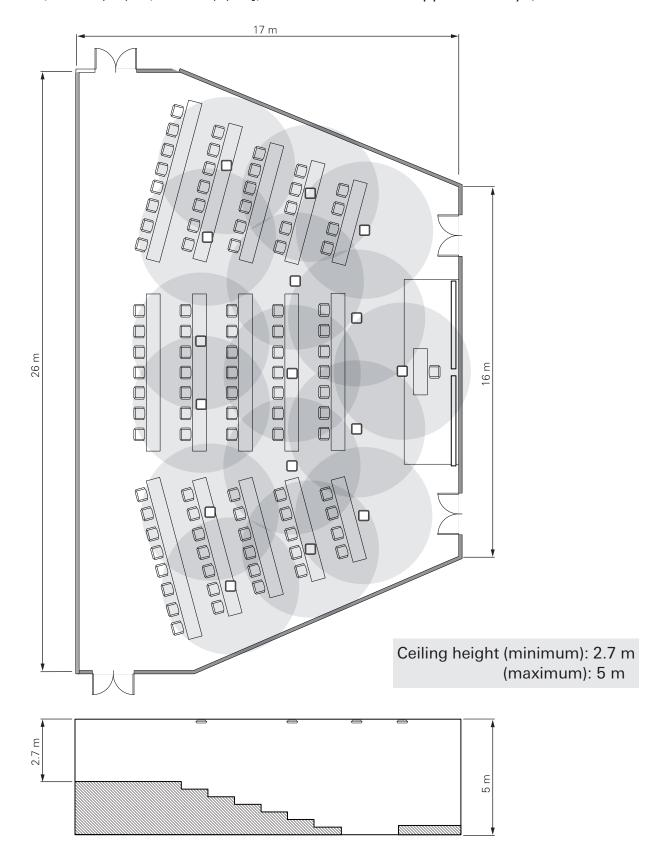
School format (maximum 16 units) [W: 20 m, D: 20 m, H: 2.7 m], transmission area: approximately  $\phi$ 6 m
