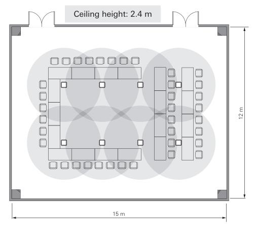
Long U shape desks [W: 18 m, D: 12 m, H: 2.7 m], transmission area: approximately  $\phi$ 6 m
