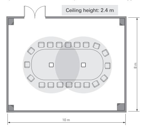
Square shape (small) [W: 12 m, D: 8 m, H: 2.4 m], transmission area: approximately  $\phi$ 5 m
