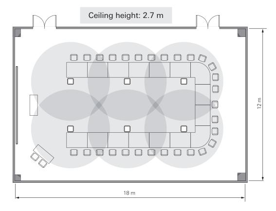
Long U shape + desks on both sides [W: 18 m, D: 12 m, H: 2.4 m], transmission area: approximately  $\phi$ 5 m
