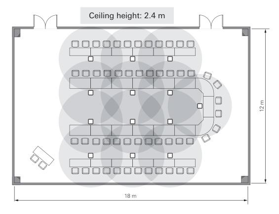
V shape [W: 15 m, D: 12 m, H: 2.7 m], transmission area: approximately  $\phi$ 6 m
