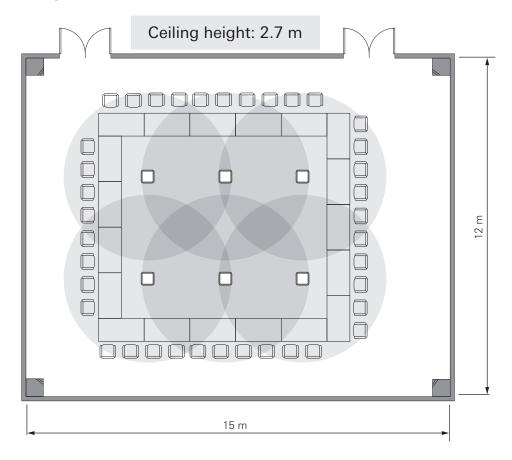
U shape + back area seats [W: 15 m, D: 12 m, H: 2.4 m], transmission area: approximately  $\phi$ 5 m
