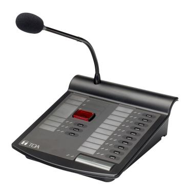
VX-100RM-EA is an IP PoE Remote Microphone.VX-100RM-EA Remote Microphone is used for general and emergency broadcast. It is equipped with 10 function switches that can be used to select individual zones or zone groups a covered switch and corresponding indicators. The optional RM-110VX-EA Remote microphone extension permits switches and indications to be expanded in 10-piece units.
