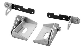
The HY-WM2WP is used exclusively to mount the HX-5 series speaker system closely to a wall or ceiling. The bracket helps to achieve clearer sound reproduction by minimizing phase interference generated by sound waves reflecting from walls or ceilings. This bracket is designed for outdoor use.
