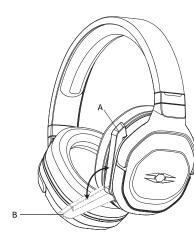
Rotate microphone upward to "A" for mute status. Rotate microphone downward to "B" for mute status.
